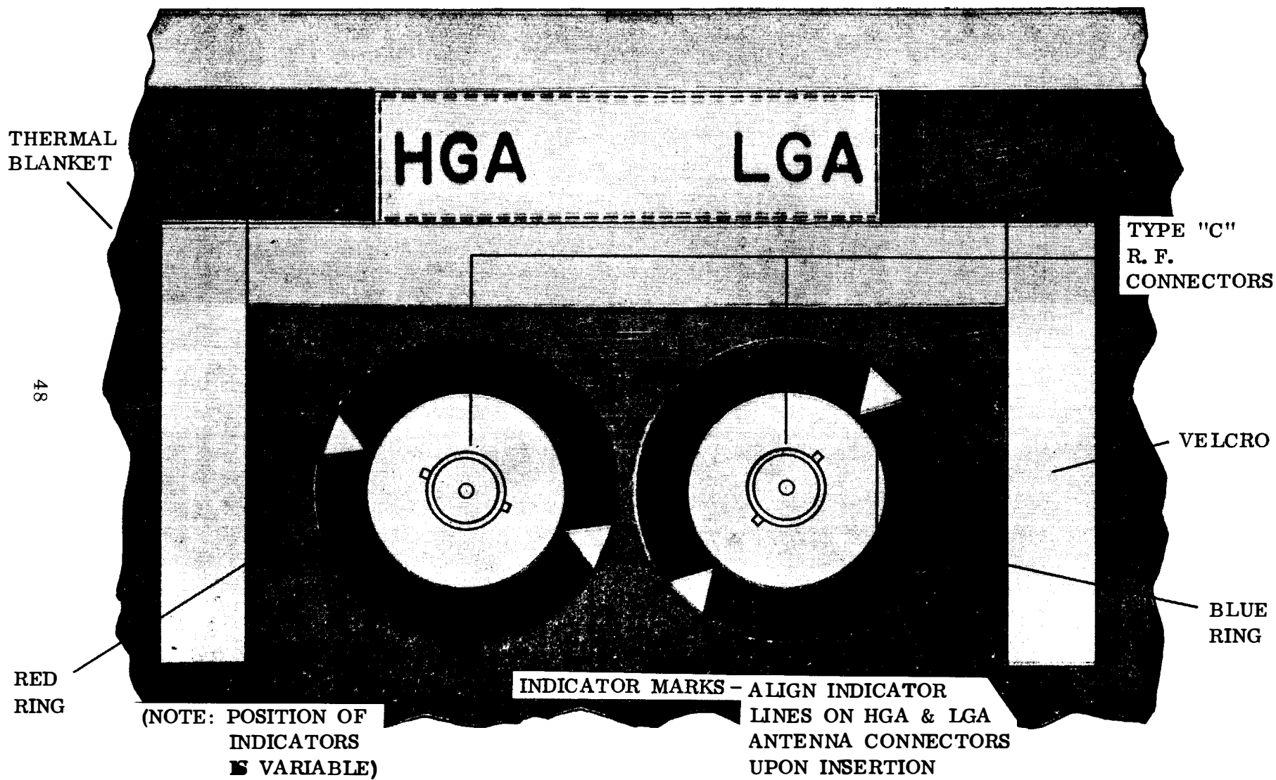
Figure 4-15. LCRU HGA & LGA Antenna Connector Inlet
