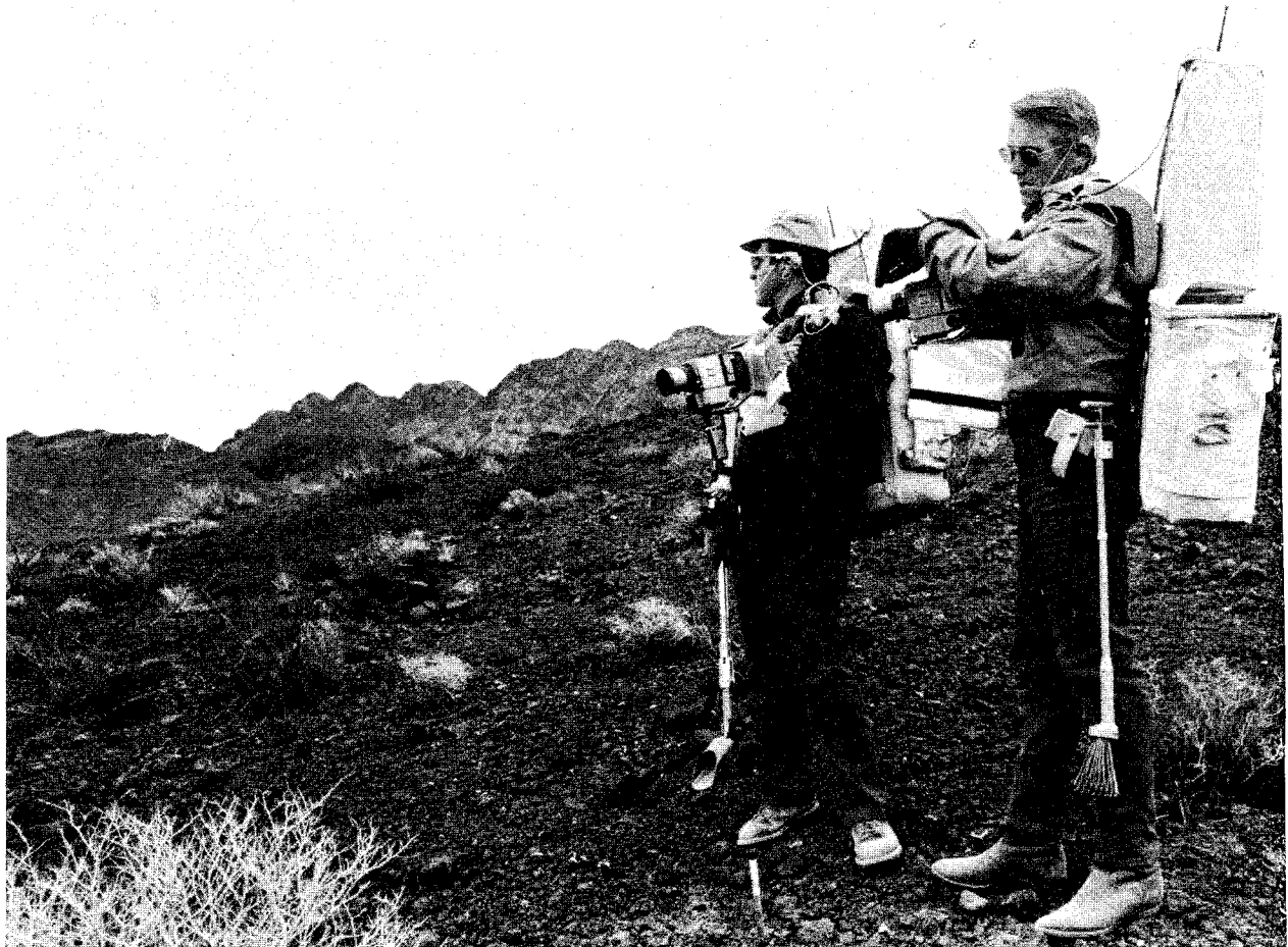
FIGURE 99.—Astronauts Schmitt and Cernan. Notice that sampling tools, like the ones to be used on the Moon, are used during the practice exercises. Each astronaut carries a Hasselblad camera, sample bags, cuff checklists, and simulated backpacks. Schmitt carries a scoop and Cernan carries tongs. NASA PHOTO 8-72-30170.
