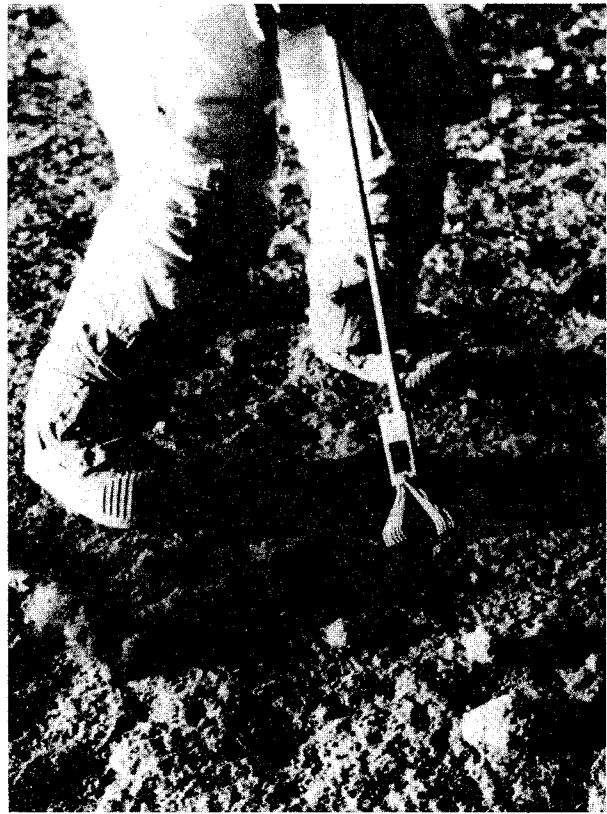
FIGURE 46.—Tongs shown in use on Apollo 12 to collect a small rock. NASA PHOTO S-71-31075.
