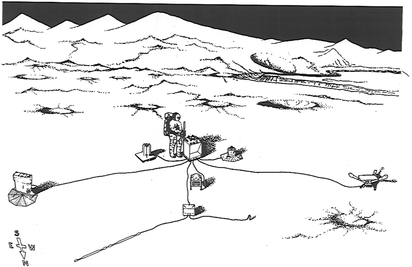
FIGURE 18.—General layout of the ALSEP. The sizes of the astronaut, equipment, and lunar features are drawn to different scales. Locations are shown in true relation to the surface features of the Moon.
