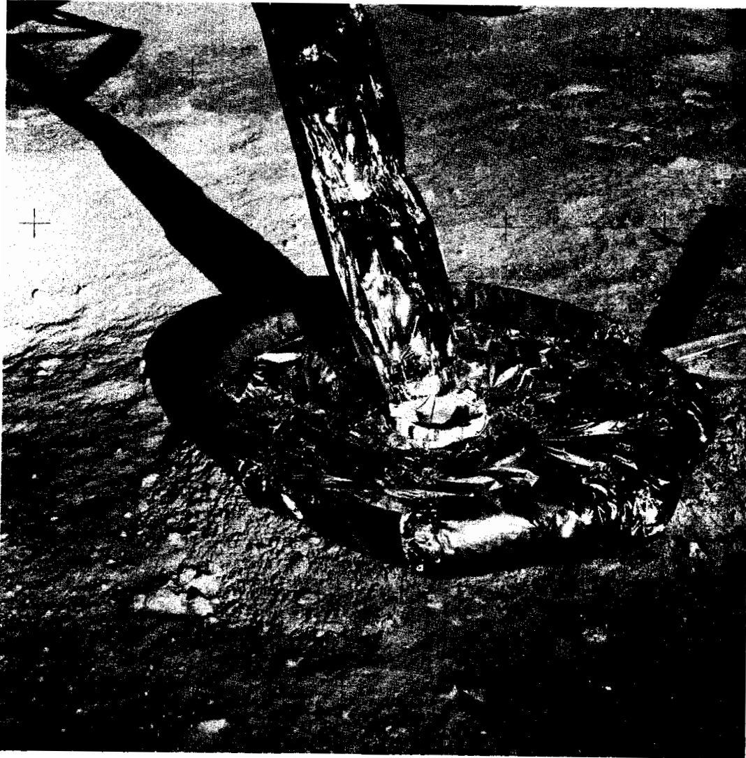
Figure 11-16.- Interaction of the minus Z footpad with lunar surface .
