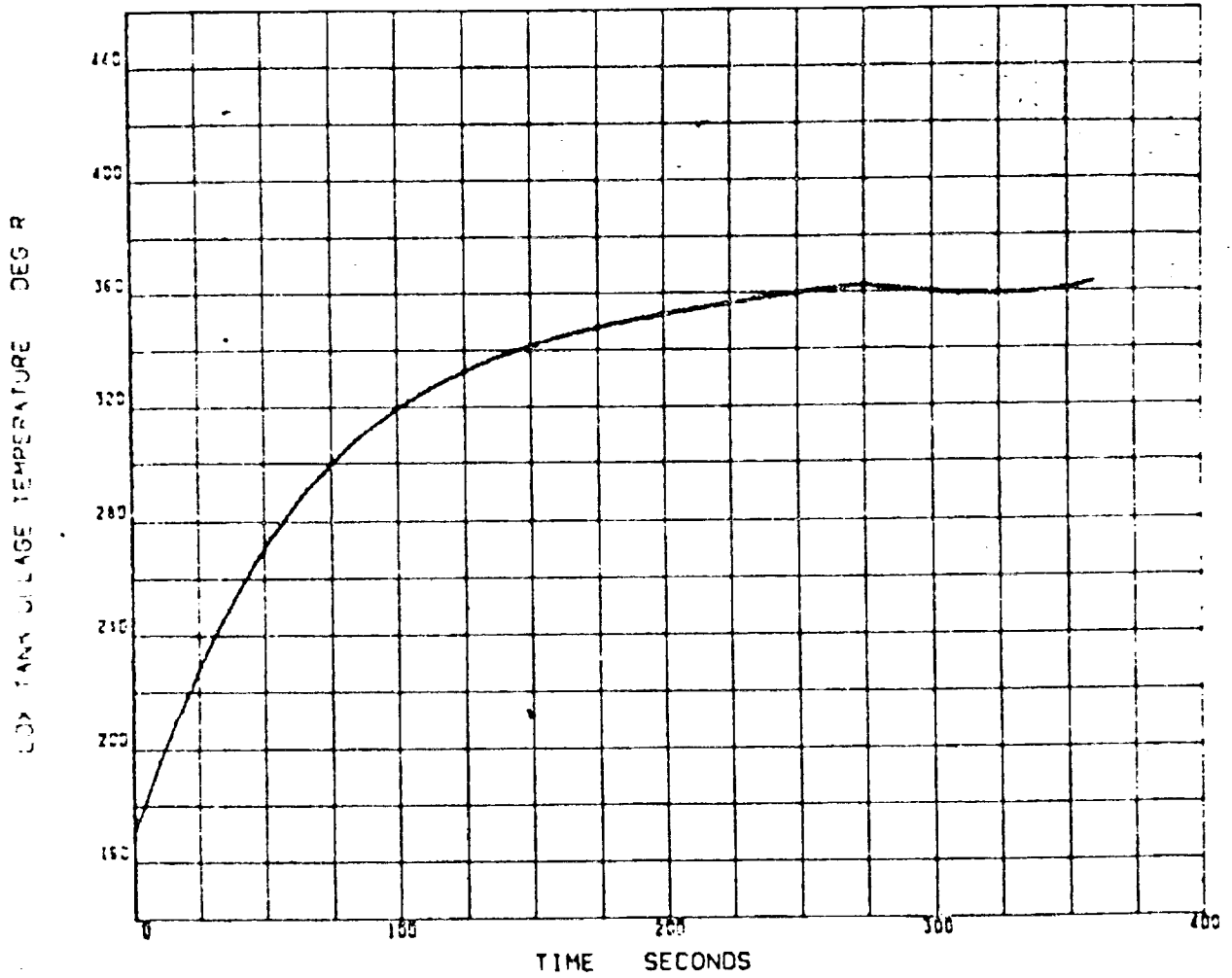
FIGURE 4-18 S-II LOX TANK ULLAGE TEMPERATURE
