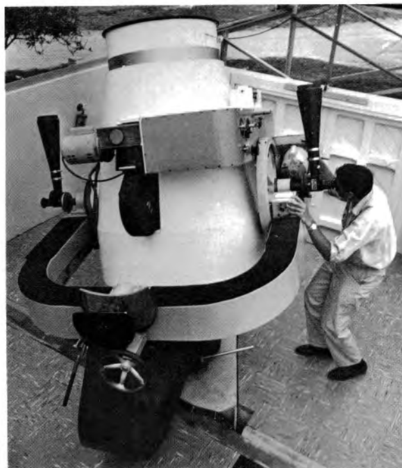
FIGURE 3-10.—Baker-Nunn satellite tracking camera and a typical installation.
