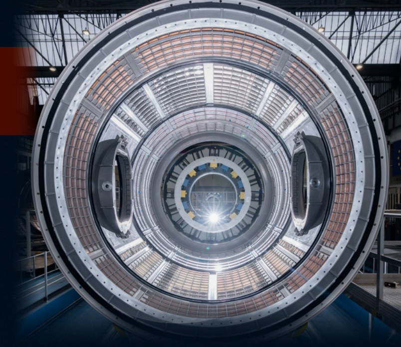
The primary structure of the Gateway space station's HALO (Habitation and Logistics Outpost) module following welding completion at Thales Alenia Space in Turin, Italy. Credit: Thales Alenia Space
