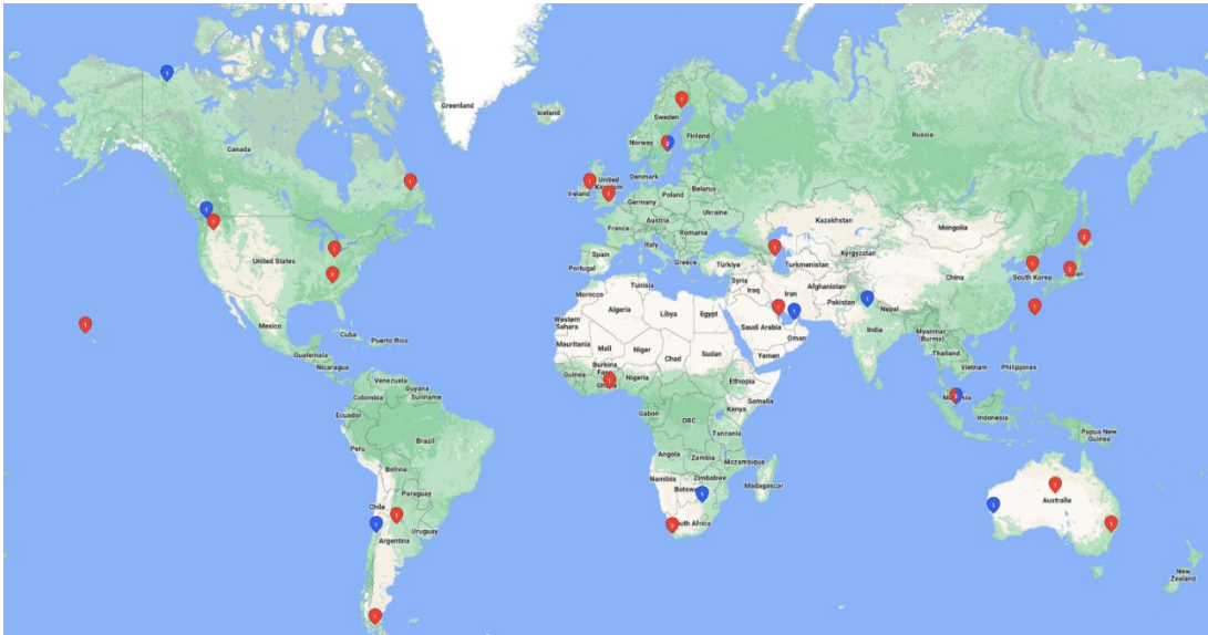
Figure 11.27: All 34 antennas on the StellarStation platform that are live (25 - red) or for which integration is planned (9 - blue). Credit: InfoStellar.
