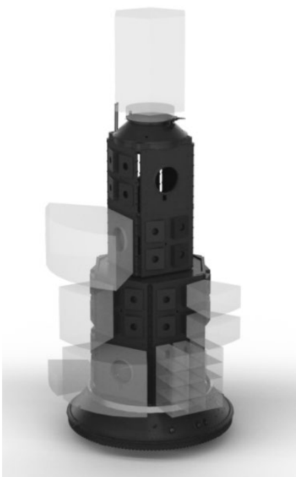
Figure 2.6: Example mission configuration using rideshare plates. Credit: SpaceX.
