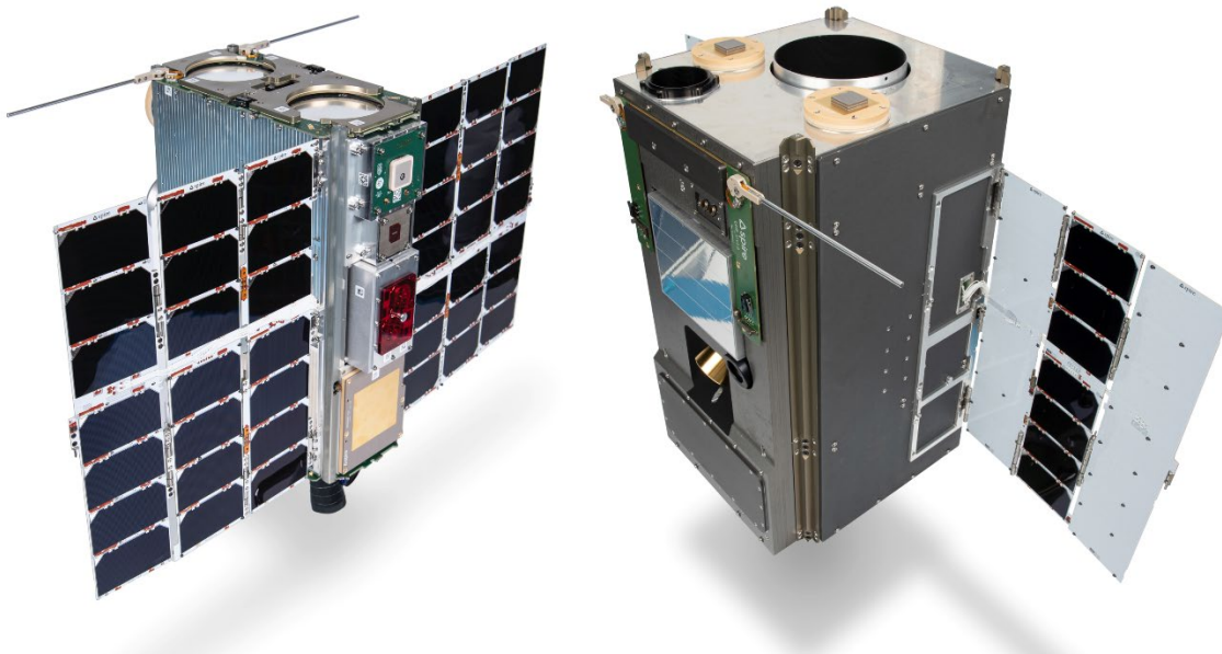
Figure 2.5: Examples of a 6U and 16U CubeSat. Credit: Spire Global.
