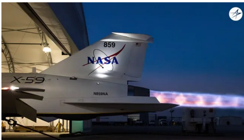
The X-59, our Quesst mission's quiet supersonic research plane, conducts afterburner engine tests at Lockheed Martin's Skunk Works facility in Palmdale, CA. Image Credit: Lockheed Martin
