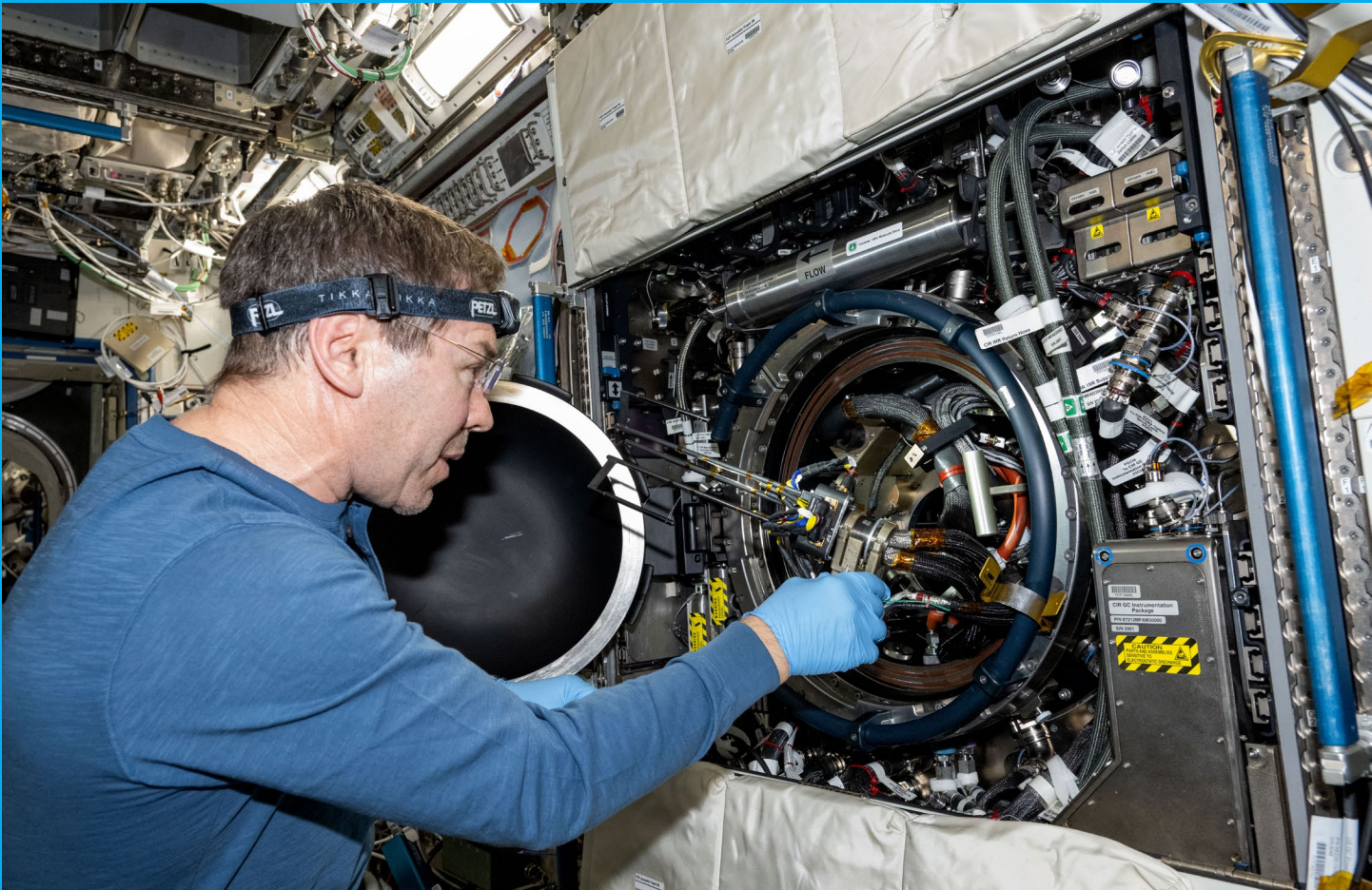
NASA astronaut and Expedition 71 Flight Engineer Mike Barratt replaces fuel bottles and other components inside the Combustion Integrated Rack located inside the International Space Station's Destiny laboratory. NASA ID: iss071e439784.
