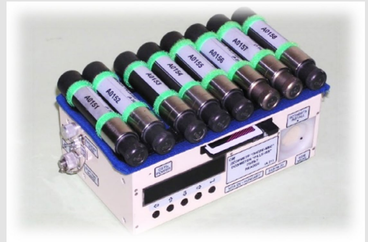
Figure 21. The Pille thermoluminescent dosimeter system including memory card and display for results. Image adopted from Pinczés, Life Sciences in Space Research .
