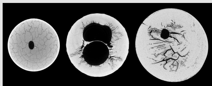
Figure 25. Microgravity samples show fractured structures upon crystallization. Images provided by the ELF research team.
