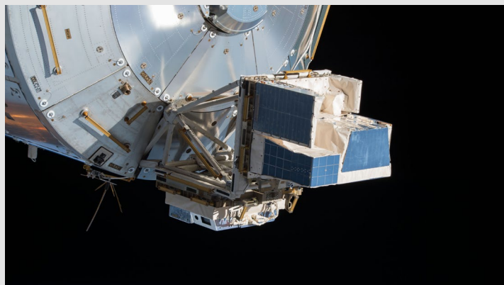
Figure 11. View of ASIM installed on the Columbus External Payload Facility. NASA ID: iss057e055411.
