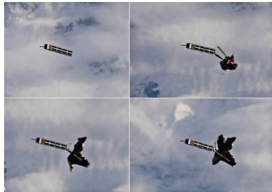
Figure 13.9: TechEdSat-10 aft-imaging captures Exo-Brake deployment July 2020. Credit: NASA.
