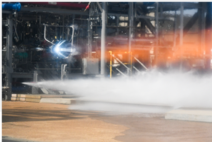
Figure 1: Hot-fire testing of a 40,000-lbf coupled thrust chamber assembly at MSFC, utilizing multi-material additive manufacturing and composite overwrap technology. (Credit: NASA)
