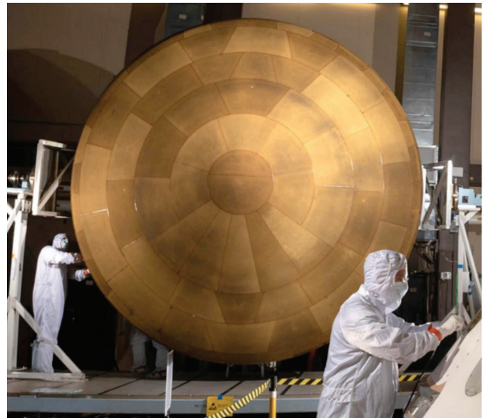
This photograph shows the Mars 2020 PICA heat shield, which protected the Perseverance rover and its descent stage during the deep space cruise to Mars and the descent through the Martian atmosphere. The image was taken at Lockheed Martin Space in Denver, Colorado, where the PICA aeroshell was integrated. Credit: NASA.
