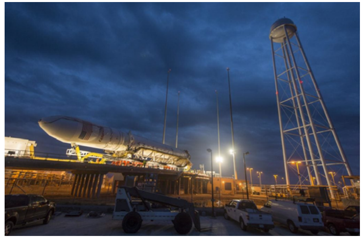
Orbital Sciences developed the Antares launch vehicle as part of the company’s COTS SAA. Originally named the Taurus II, the 131-foot rocket is capable of lifting over 11,000 pounds to LEO. This medium-class vehicle reflected the company’s philosophy of relying on proven hardware components. 234 Credit: NASA/Brea Reeves.
