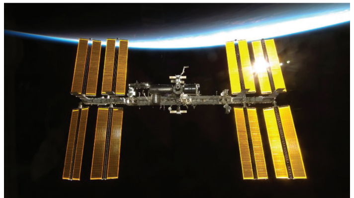
With a backdrop of Earth's horizon and the blackness of space, the ISS is featured in this image photographed by an STS-130 crew member as the space shuttle Endeavor and the station approach each other during rendezvous and docking activities. Docking occurred at 11:06 p.m. (CST) on February 9, 2010, delivering the Tranquility node and its cupola. Credit: NASA.
