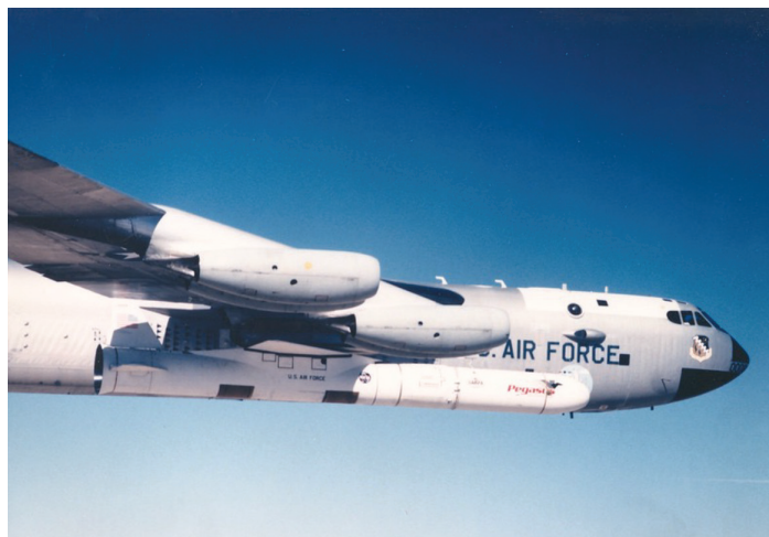
This image shows a Pegasus being carried to altitude by a NASA-obtained B-52 on April 5, 1990. An air-launched, three stage, all solid-propellant, three-axis stabilized vehicle, the Pegasus was designed to put a 400- to 1,000-pound payload into LEO. Credit: NASA on the Commons/Flickr.
