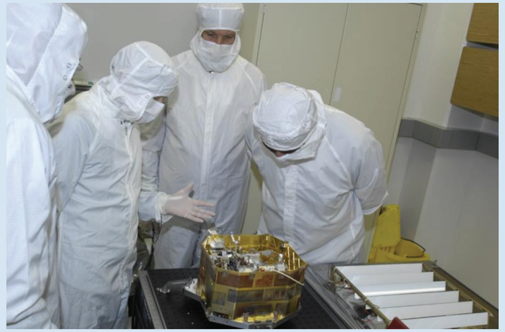
The Moon Mineralogy Mapper imaging spectrometer, an instrument on India's Chandrayaan-1, during development at NASA's JPL. Credit: NASA/JPL-Caltech.
