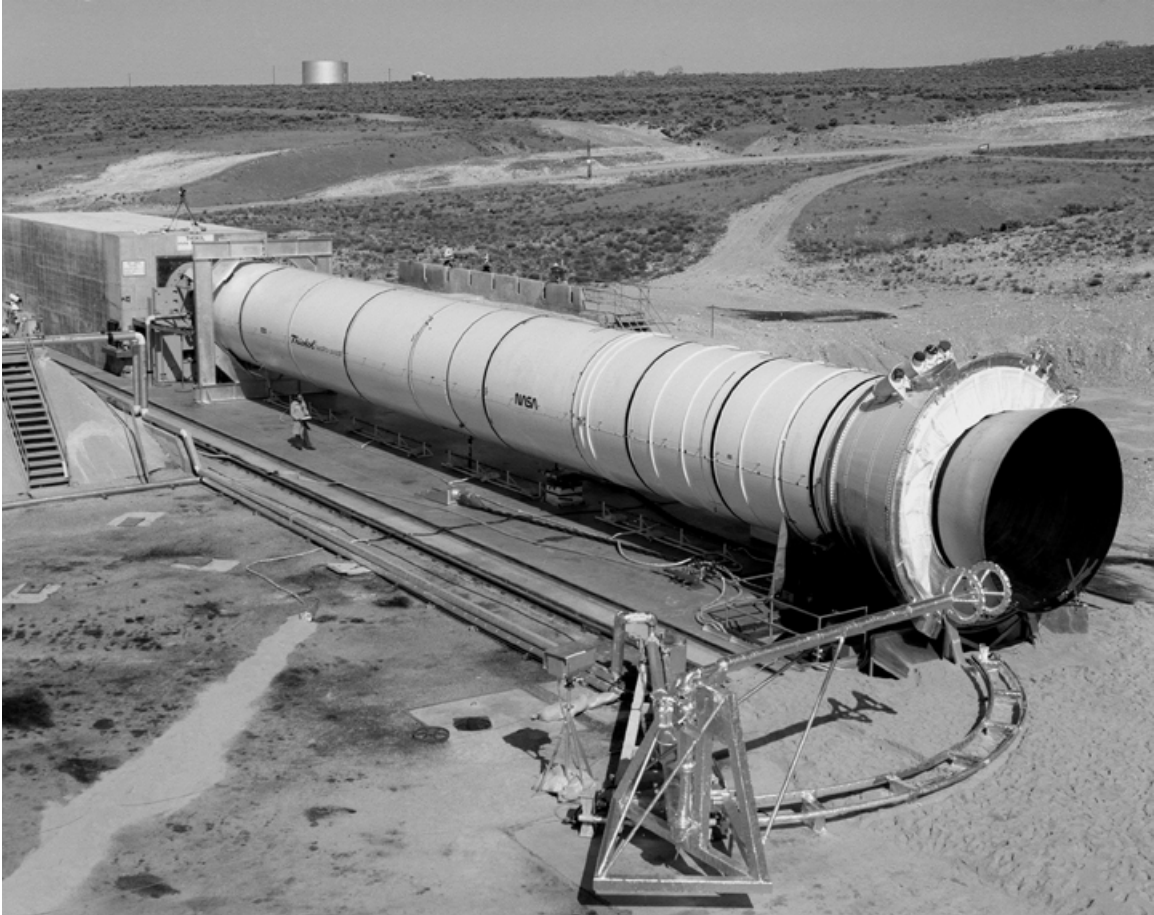
Figure No. E-2. SRB Qualification Motor-1 (QM-1) in test stand at Morton Thiokol facility at Wasatch, Utah, July 13, 1979.
