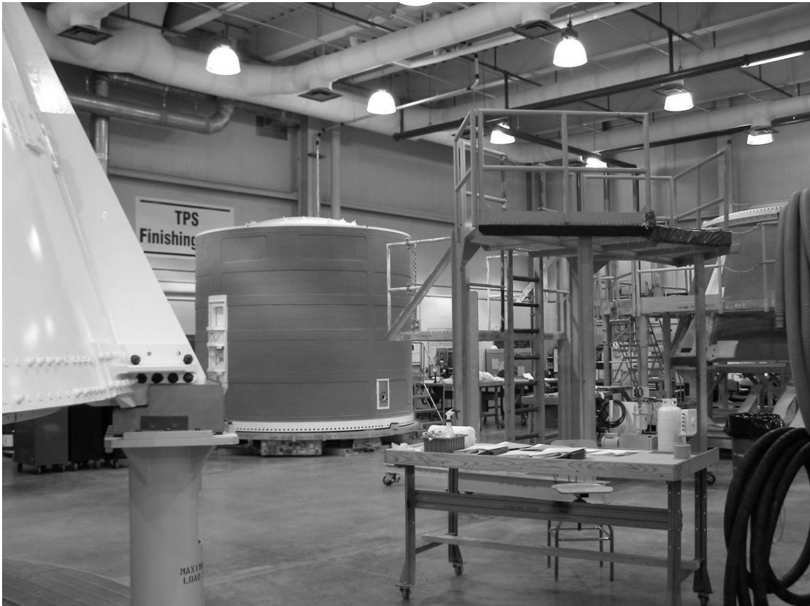
Figure No. E-46. SRB forward skirt in the SRB ARF cure area. Source: Archaeological Consultants, Inc., 2006.
