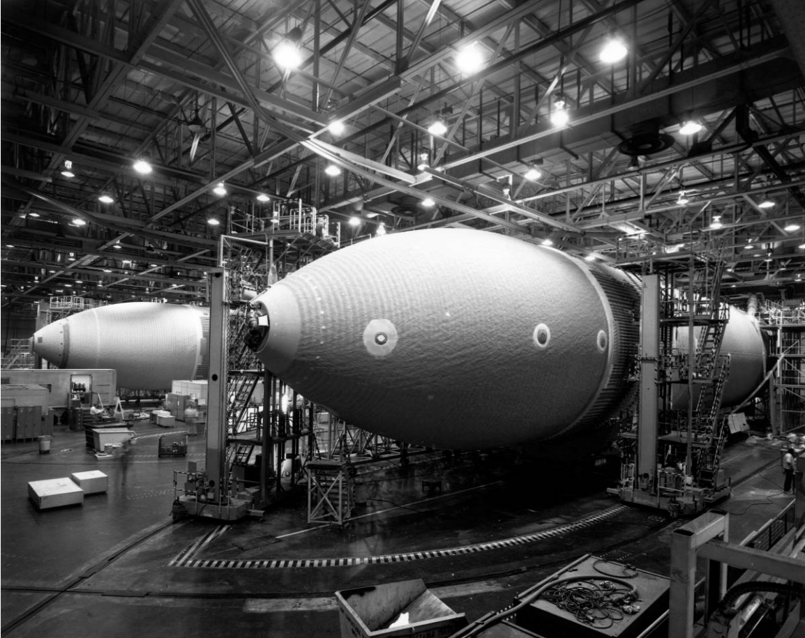
Figure D-5. A Standard Weight Tank (foreground) and a Lightweight Tank (rear) in final assembly at MAF, date unknown.
