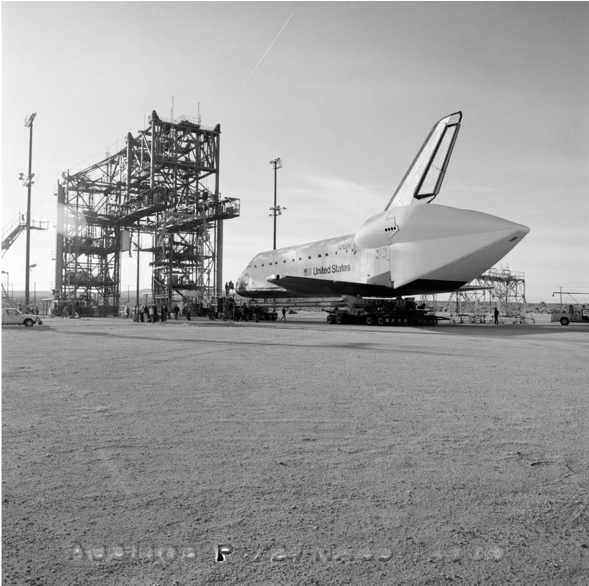
Figure B-60. Discovery ready to be positioned in the Mate-Demate Device at DFRC for attachment to the SCA for delivery to KSC, November 5, 1983. Source: NASA, Johnson Space Center Image Repository, JSC2010-00016.
