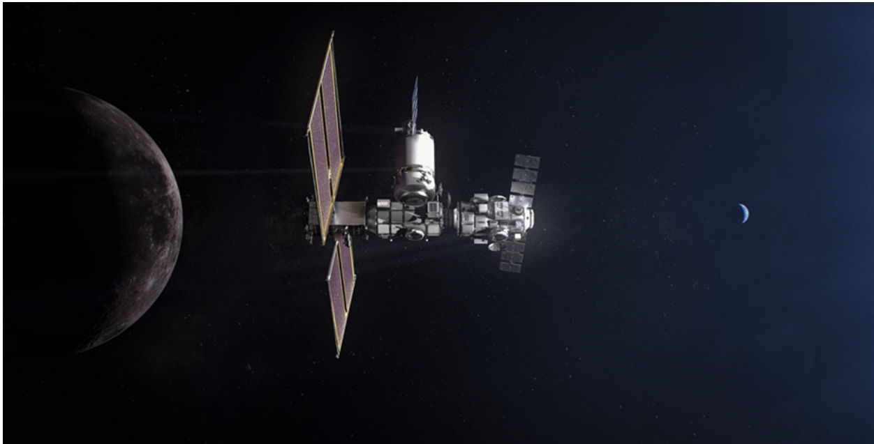
Figure 3-2. Gateway Crew-Capable Configuration
