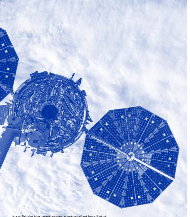
Image: This view from the main window on the International Space Station's cupola shows Northrop Grumman's Cygnus space freighter in the grip of the Canadarm2 robotic arm moments before its release.
