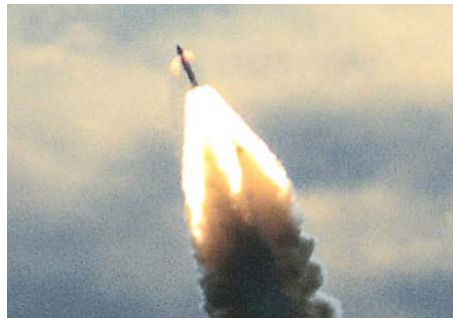
The Orion launch abort system successfully flew through brief periods of instability. Known instabilities and risks were evaluated prior to flight using best practices.
