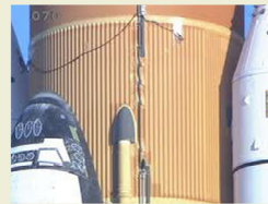
External tank stringer
