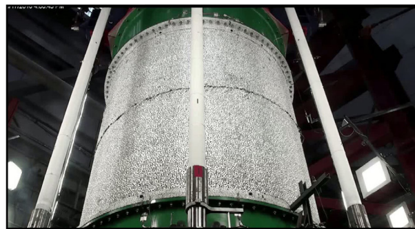
Sandwich composite test article showing material failure that occurred as a result of global buckling.
