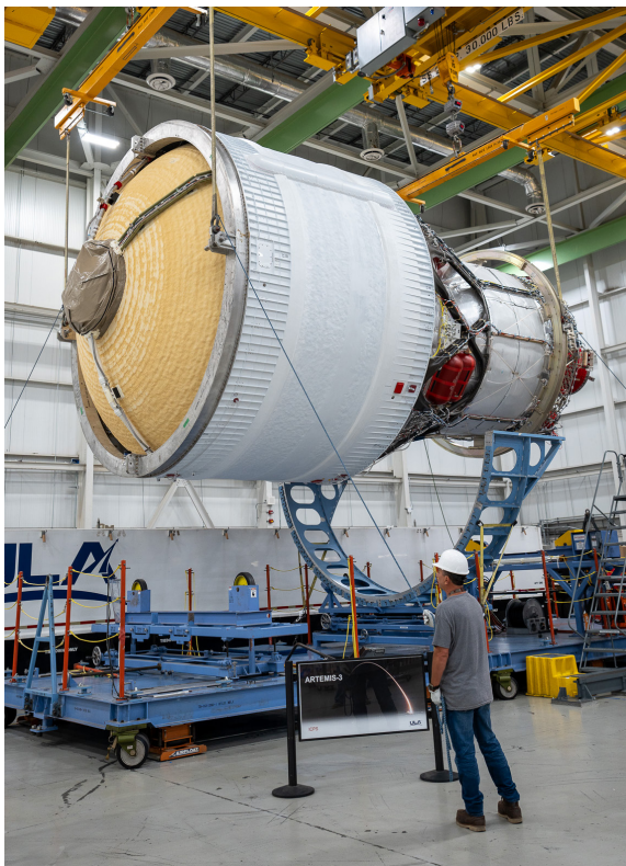
The interim cryogenic propulsion stage (ICPS), a modified United Launch Alliance Delta Cryogenic Second Stage, provides 24,750 lbs. of thrust for in-space propulsion for the Block 1 crew and cargo vehicles.
