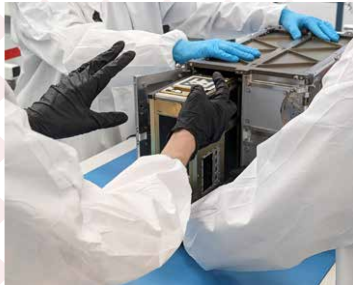
A NASA engineer installs the agency's CubeSat R5 Spacecraft 4 (R5-S4) into the dispenser at Firefly Aerospace's Payload Processing Facility at Vandenberg Space Force Base in California ahead of the company's Demonstration 2 launch for NASA. Photo Credit: NASA/Jacob Nunez-Kearney
