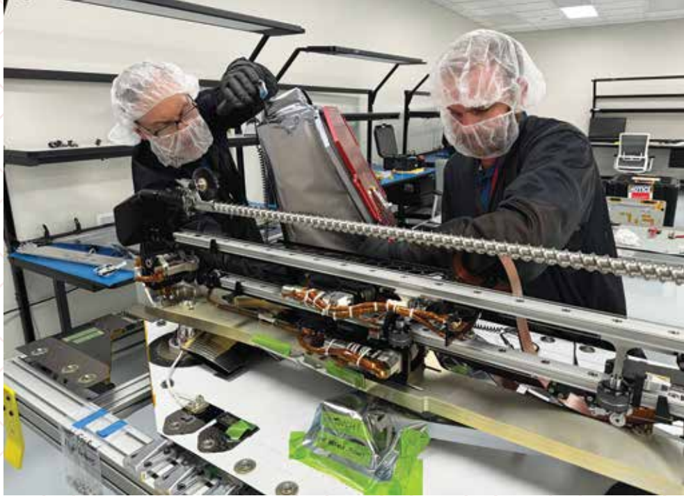
Teams with NASA and Intuitive Machines work together to integrate MSOLO (Mass Spectrometer Observing Lunar Operations) onto a lunar lander for the PRIME-1 (Polar Resources Ice Mining Experiment-1) flight. Photo credit: NASA
