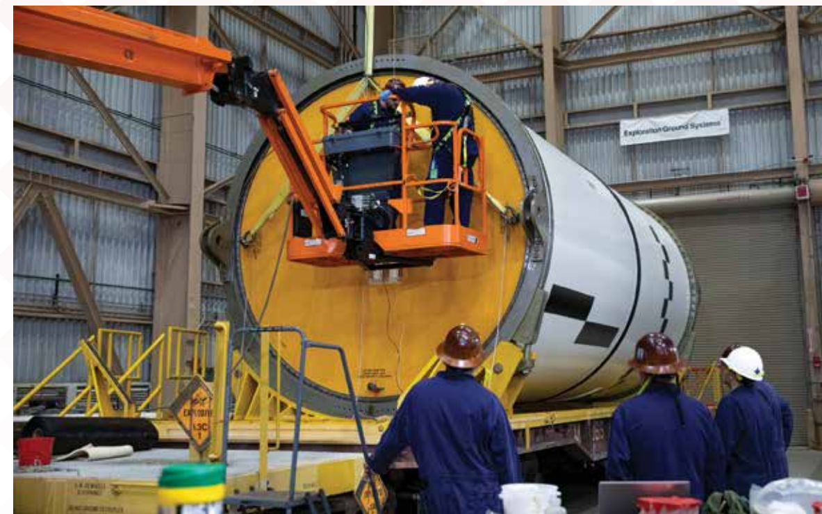
Engineers and technicians process the right forward center segment of the SLS (Space Launch System) solid rocket boosters for the Artemis II mission inside the Rotation, Processing and Surge Facility (RPSF) at NASA's Kennedy Space Center in Florida by removing the yellow cap and inspecting propellant on Nov. 27, 2023. Photo credit: NASA/Kim Shiflett
