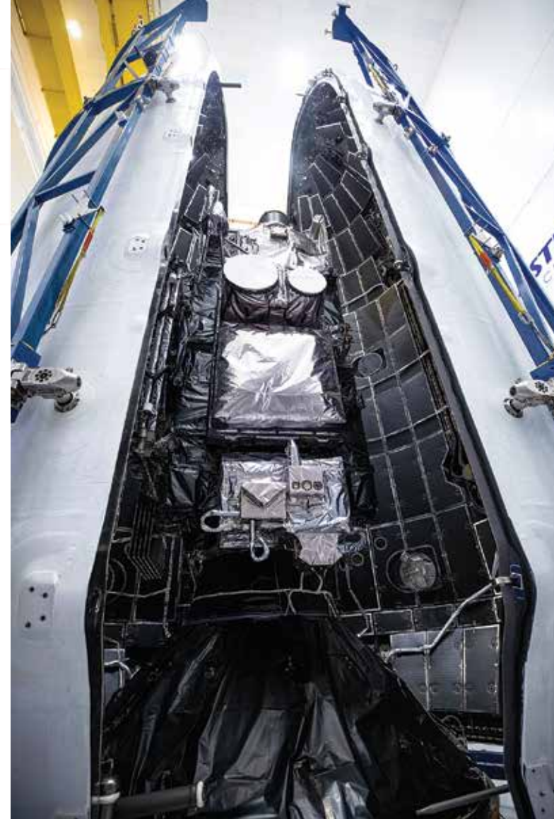
Technicians prepare NOAA's GOES-U satellite for encapsulation inside payload fairing halves at the Astrotech Space Operations Facility in Florida. Photo Credit: NASA/Ben Smegelsky
