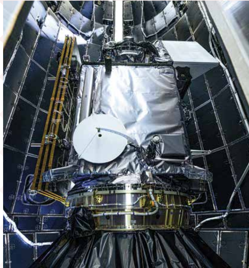
Above: NASA and SpaceX technicians safely encapsulate NASA's PACE (Plankton, Aerosol, Cloud, ocean Ecosystem) spacecraft in SpaceX's Falcon 9 payload fairings on Jan. 30, 2024, at the Astrotech Space Operations Facility near the agency's Kennedy Space Center in Florida. Photo credit: NASA/Denny Henry
