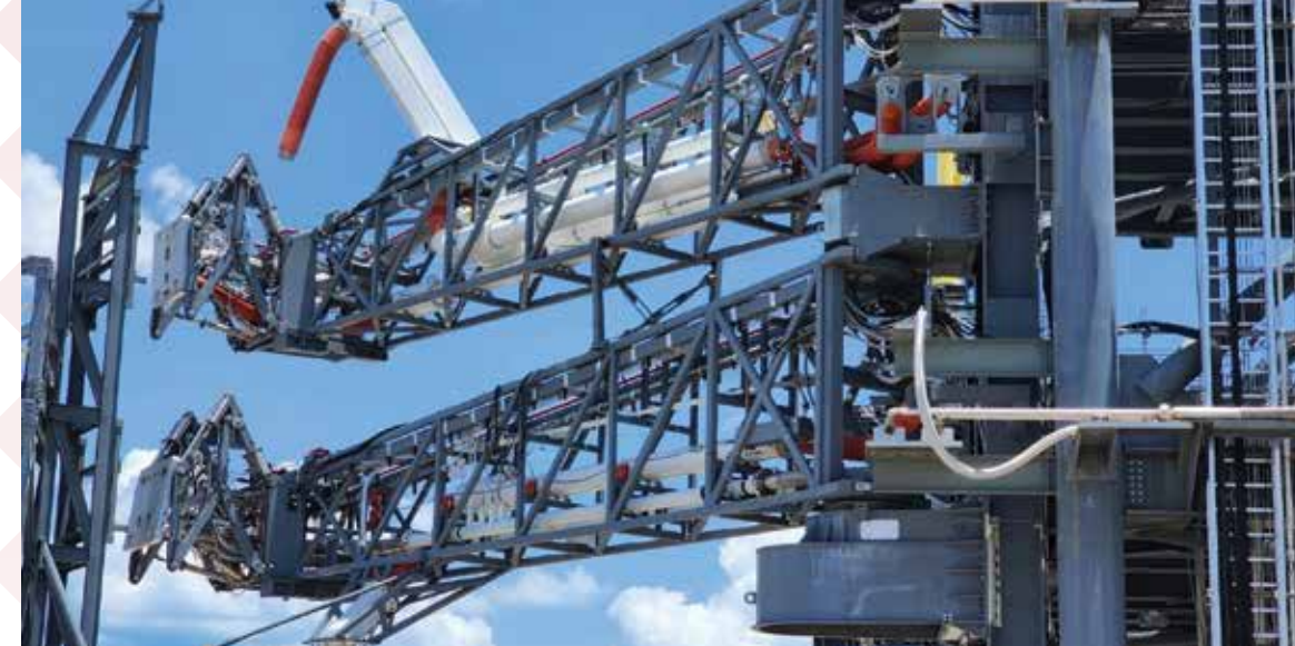
Teams work on the next phase of exploration upper stage umbilical testing at the Launch Equipment Test Facility. The umbilical is part of mobile launcher 2, designed to support the SLS (Space Launch System) Block 1B configuration and provide liquid hydrogen and oxygen to the exploration upper stage. Photo credit: NASA
