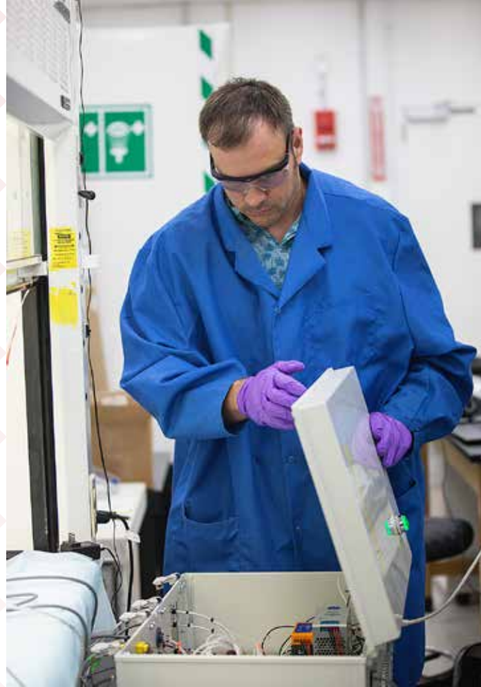
Beau Peacock, software engineer, conducts testing of the Volatile Monitoring Oxygen Measurement Subsystem (VMOMS) for Molten Regolith Electrolysis (MRE) inside a laboratory in the Neil A. Armstrong Operations and Checkout Building at NASA's Kennedy Space Center in Florida on April 19, 2024. The high-temperature electrolytic process aims to extract oxygen from simulated lunar regolith which will be critical to the agency's Artemis campaign. Photo Credit: NASA/Isaac Watson
