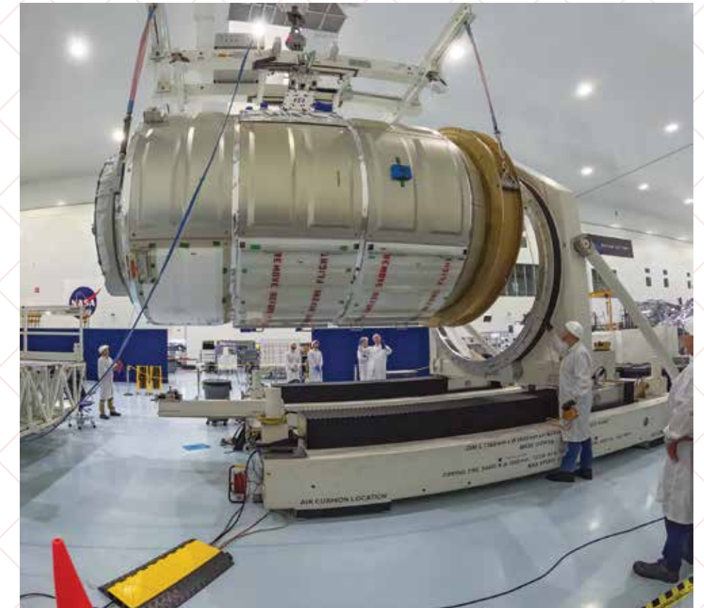
The Northrop Grumman Cygnus spacecraft's pressurized cargo module for the company's 21st commercial resupply mission is moved by a crane inside the Space Systems Processing Facility at NASA's Kennedy Space Center in Florida on June 1, 2024, as prelaunch processing operations continue. Photo credit: NASA/Glenn Benson
