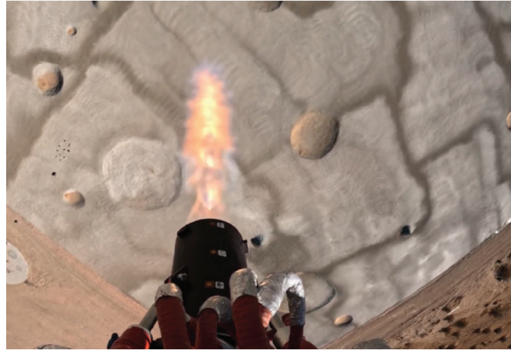
Astrobotic’s Xodiac lander flies over its simulated lunar surface during the Nov. 14 test of the company’s advanced lidar hazard detection system. Credits: Astrobotic
