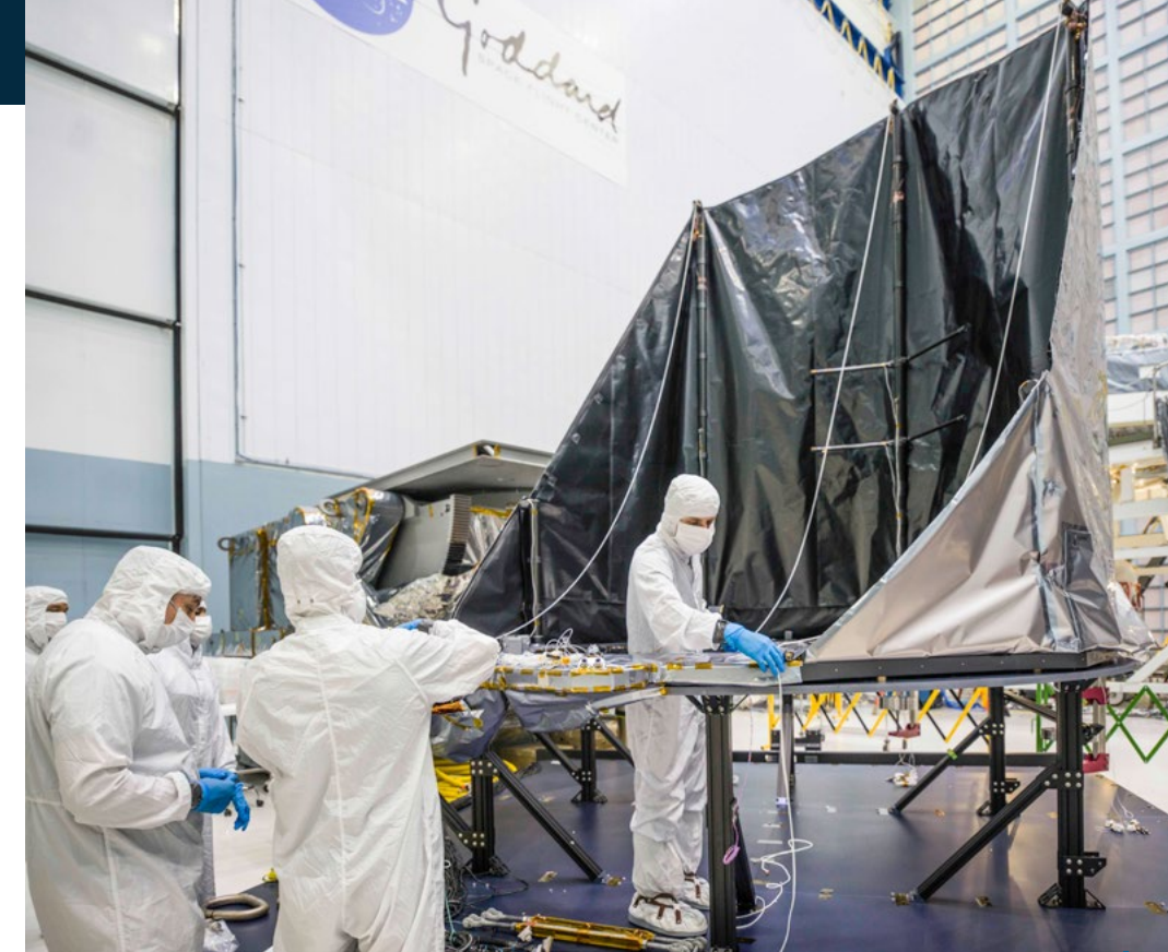
After a successful test deployment at NASA's Goddard Space Flight Center in Greenbelt, MD, clean room technicians inspect the Deployable Aperture Cover for NASA's Nancy Grace Roman Space Telescope. CREDIT: NASA/CHRIS GUNN
