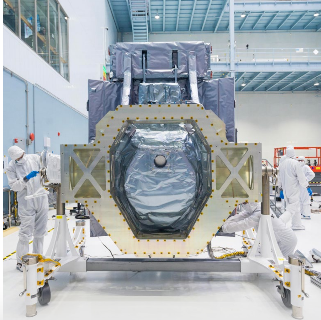
This photo shows the Wide Field Instrument arrives at the big clean room at NASA's Goddard Space Flight Center. About the size of a commercial refrigerator, this instrument will help astronomers explore the universe's evolution and the characteristics of worlds outside our solar system. Unlocking these cosmic mysteries and more will offer a better understanding of the nature of the universe and our place within it. CREDIT: NASA/CHRIS GUNN
