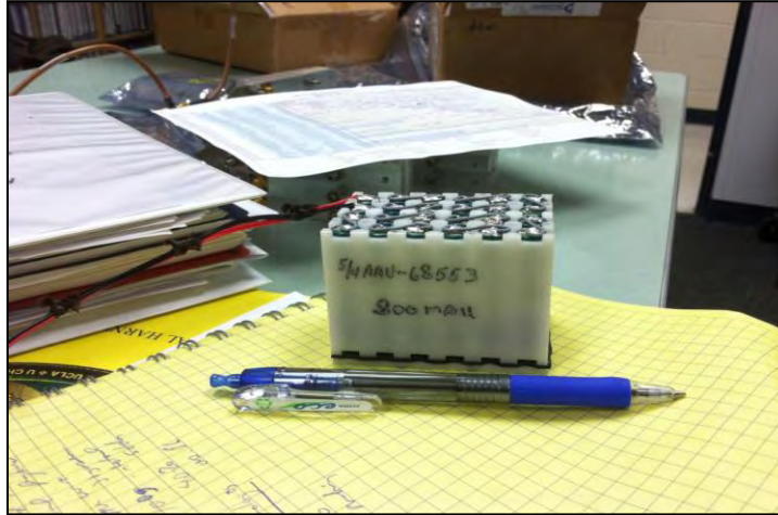
Figure 4–14. Typical Rocket Motor Ignition Battery Pack
