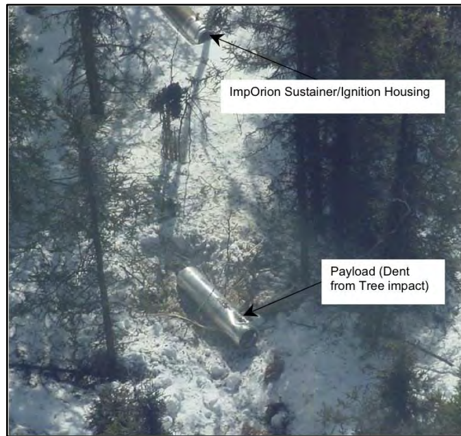
Figure 4–5. Impact Site of Failed Terrier-Improved Orion from March 2003
