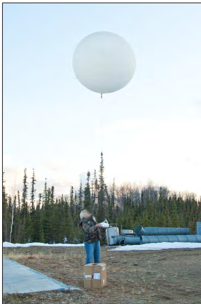
Figure 2–26. Launching a GPS Radiosonde Balloon from PFRR
