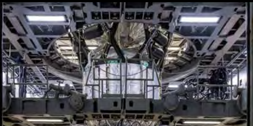
Interim cryogenic propulsion stage final testing and checkout
