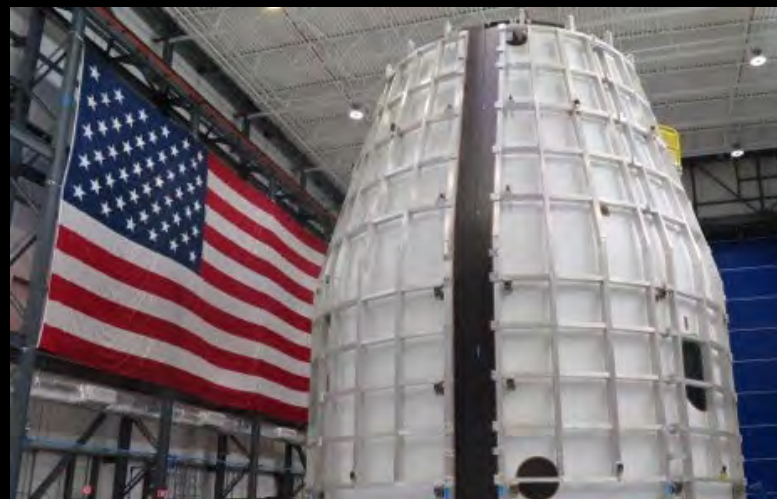
All four universal stage adapter structural qualification article panels are aligned and loaded on Vertical Assembly Tool
