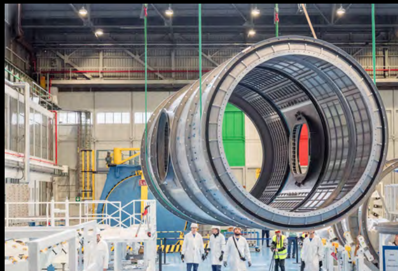
Gateway Habitation and Logistics Outpost (HALO) undergoes stress testing at Thales Alenia Space facility on June 10
