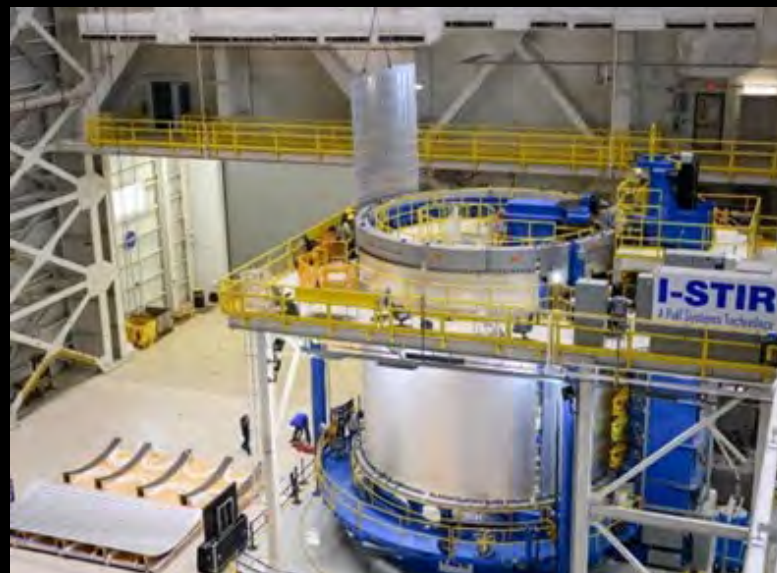
Liquid hydrogen tank for core stage in progress
