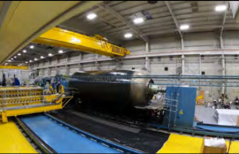
Trial Booster Obsolescence and Life Extension (BOLE) composite case winding toward SLS Block 2
