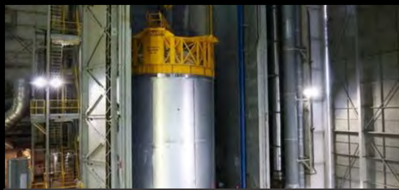
Core stage liquid oxygen tank at Vertical Assembly Center at Michoud
