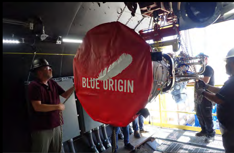
Blue Moon HLS's in-space engine BE-7 hotfire test in a vacuum cell at Edwards Air Force Base
