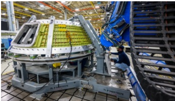
Technicians from Orion prime contractor Lockheed Martin weld together three cone-shaped panels on Orion's crew module pressure vessel for the Artemis V mission. (NASA/MSFC/MAF)
