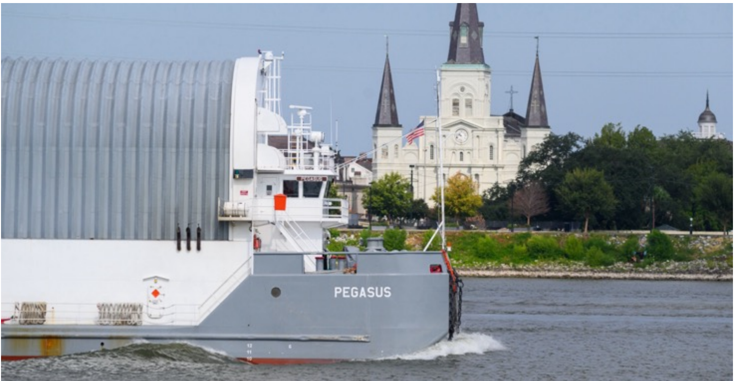
The Pegasus barge, originally used during the Space Shuttle program, has been redesigned and extended to accommodate the SLS rocket's 212-foot-long core stage — the backbone of the rocket. (NASA/MSFC/MAF)
