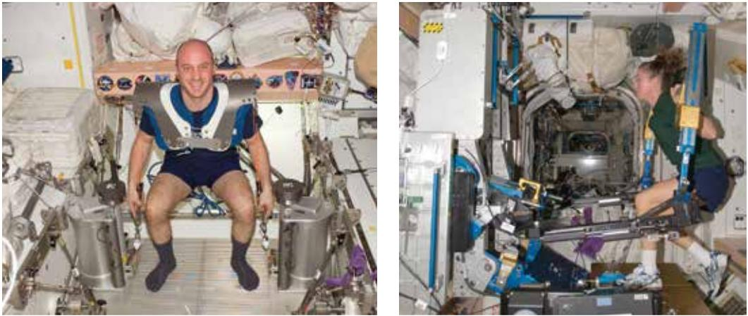
Figure 24. Garrett Reisman shown using the interim Resistance Exercise Device (iRED, left), while Sandy Magnus is shown using the Advanced Resistance Exercise Device (ARED, right) on ISS. The iRED was launched in 2000 with the first ISS crew, and the ARED replaced it in late 2008.
