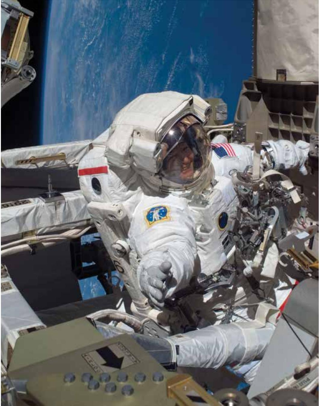
*Expedition 16 Commander Peggy Whitson pauses for a photo while working on the S5 Truss during Bearing Motor Roll Ring Module removal and replacement operations.*
