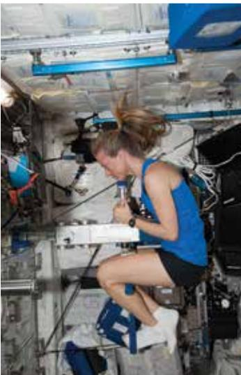
Figure 12. Karen Nyberg (left), Expedition 36 Flight Engineer, using the Space Linear Acceleration Mass Measurement Device. Tom Marshburn (right), Expedition 34 Flight Engineer, using the Body Mass Measurement Device. Photo credits: NASA.
