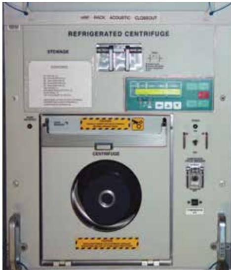
Figure 2. The refrigerated centrifuge on ISS.
