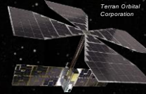
PTD-4 Pathfinder Technology Demonstrator-4 Lightweight Integrated Solar Array and anTenna (LISA-T)
