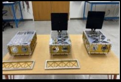
Active Thermal Architecture providing payload thermal support and setpoint thermal control for the Active Cooling for Multispectral Earth Sensors (ACMES) mission.
