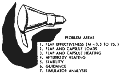
Figure 2.—One version of the "lifting" Mercury capsule being considered in 1960 for a flight-test program between the end of Mercury and the start of a manned circumlunar program. (STG, "Guidelines for Advanced Manned Space Vehicle Program," June 1960, p. 53)
