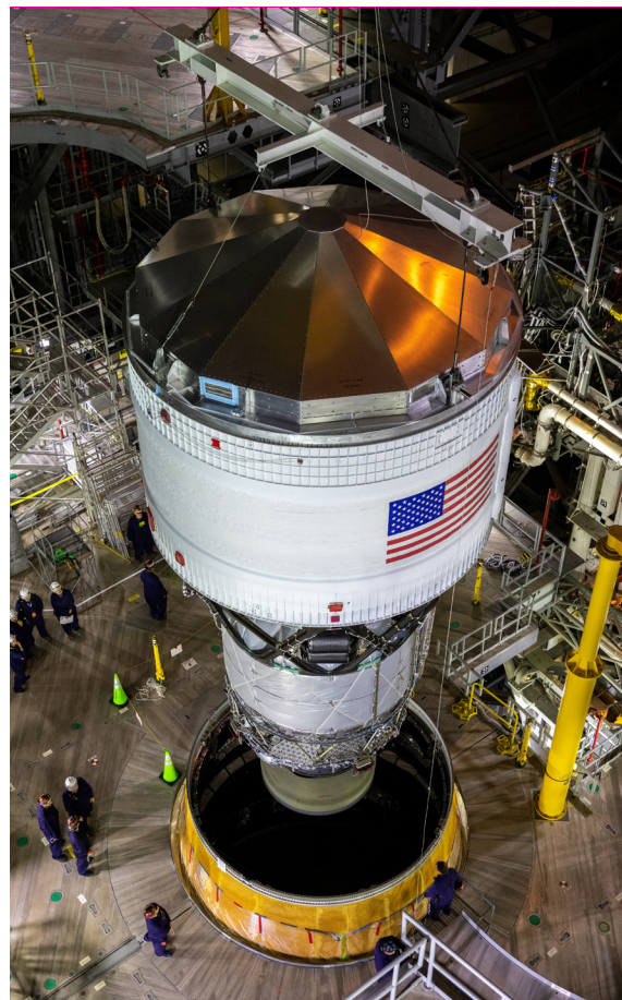
The LVSA connects the mega rocket's core stage to the interim cryogenic propulsion stage, partially enclosing it and protecting its avionics and electrical systems from the extreme pressures, sounds, and temperatures during launch and flight.
