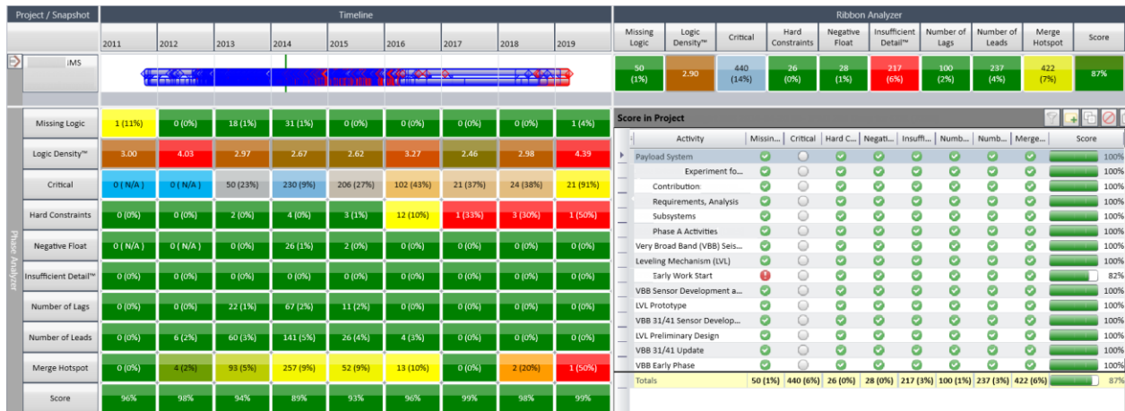
Figure 8-19. A Health Check assessment generated from the Deltek Acumen Fuse tool. A variety of Health Check Reports can be generated using the dashboards and report formats available for illustrating both built-in and custom health check metrics.
