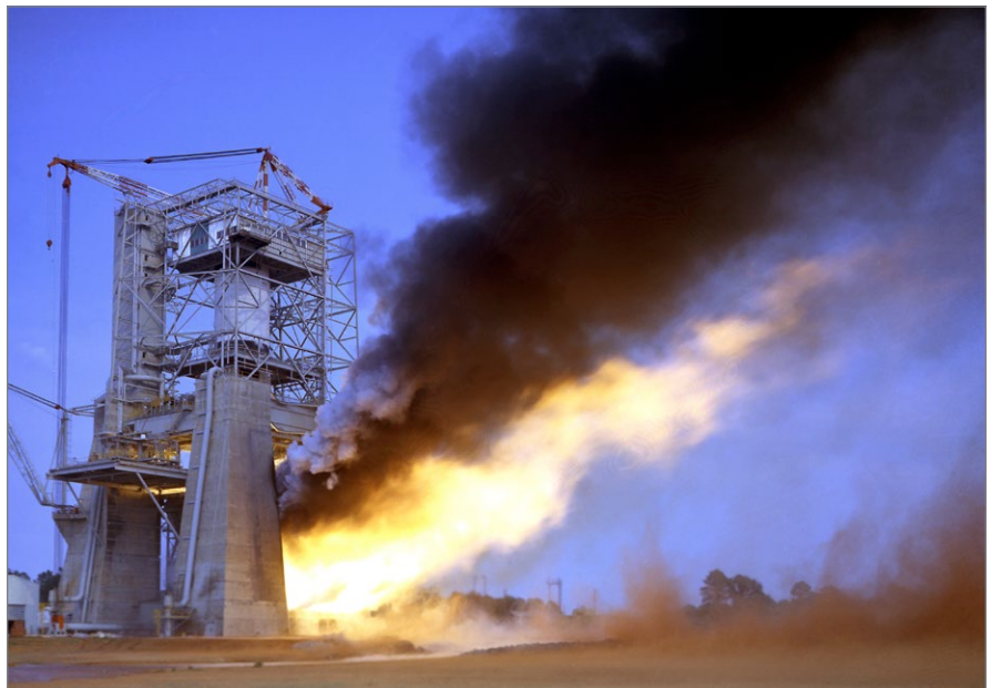
↑ All five F-1 engines for the Saturn V S-IC stage are tested at Marshall's S-IC Static Test Stand in 1965. (Photo credit: NASA)
