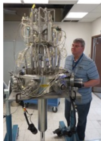
Thermal-Vacuum System Test with Depleted Uranium Core at GRC
