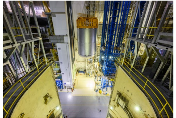
Technicians at NASA's Michoud Assembly Facility in New Orleans move the structurally complete liquid oxygen tank for the Artemis III SLS core stage after it finished welding Jan. 8. All major structures for the SLS core stage for Artemis III are now structurally complete.
