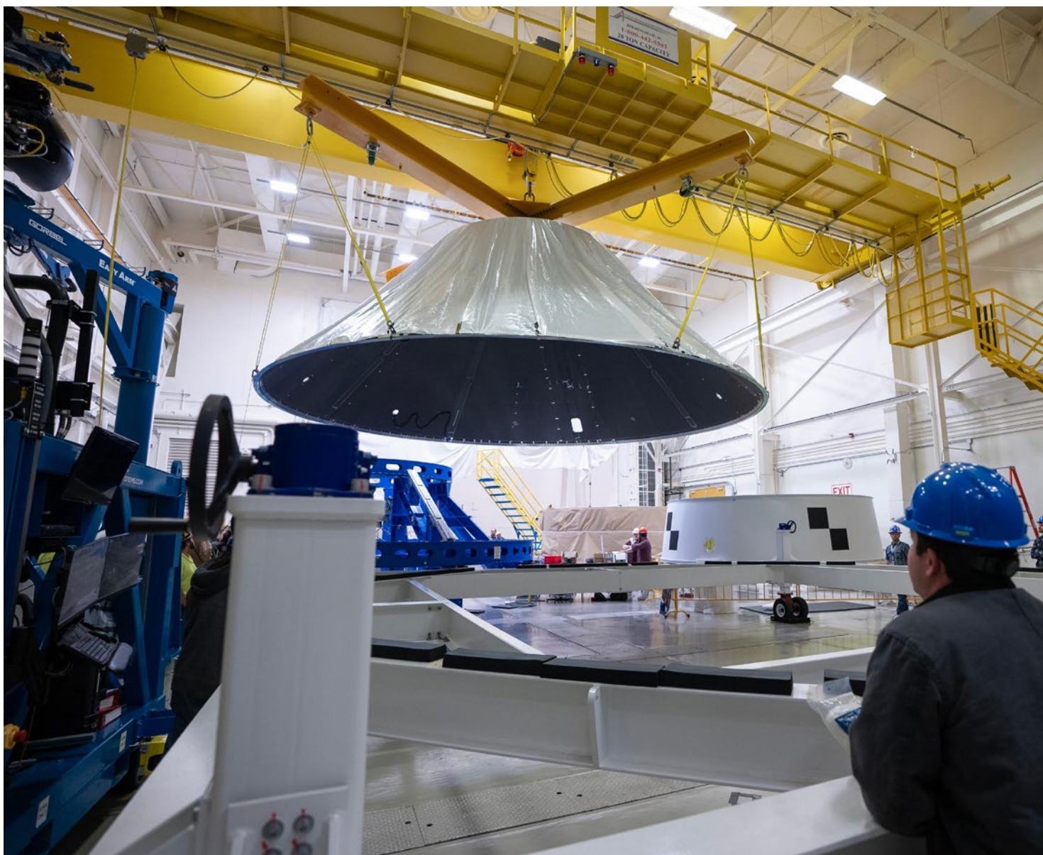
SLS Block 1B's payload adapter is lifted as part of moving the adapter to a test stand.
