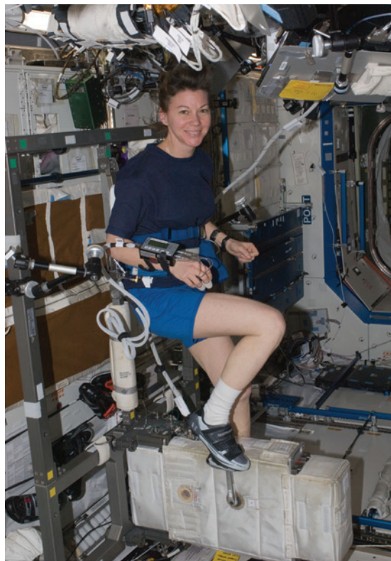
Figure 57. NASA astronaut Catherine (Cady) Coleman exercises on the Cycle Ergometer with Vibration Isolation System (CEVIS) in the U.S. Laboratory module on the ISS. Photo Credit: NASA.
