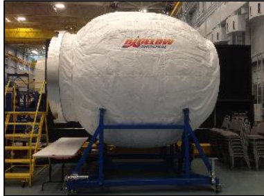
Bigelow Expandable Activity Module (BEAM): Test of inflatable module structures on ISS (JSC).
