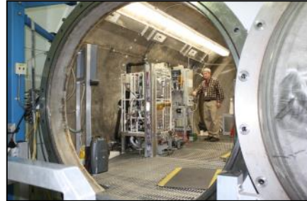
Atmosphere Resource Recovery & Environmental Monitoring: Integrated ground testing of ISS-derived life support system components (MSFC).
