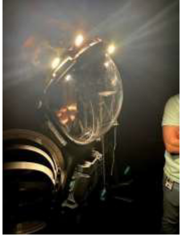
xEVA DVT Helmet Light Testing
