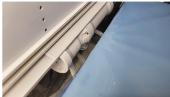
Fig. 42 Slight particle accumulation on radiator cover actuator and on edge of radiator
