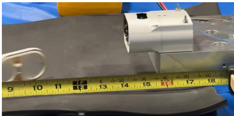
Fig. 38 Lens deploying from camera body after HDRM actuation.
