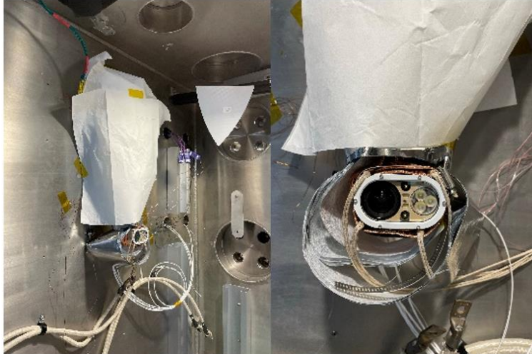
Fig. 34 IPEX camera installed in the ASSIST chamber.
