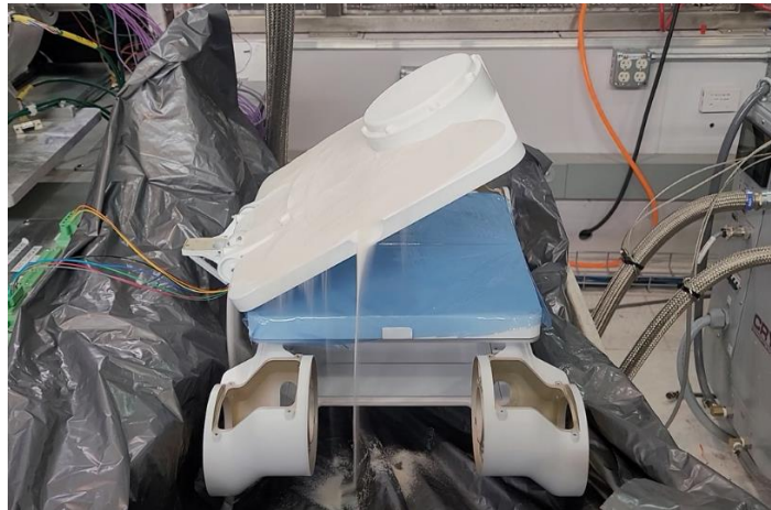
Fig. 41 Silica sand flowing off radiator cover during testing.
