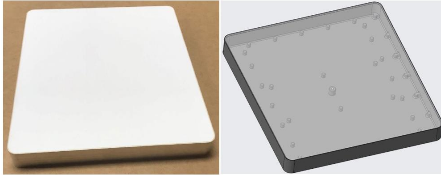
Fig. 47 PCM hardware on left, PCM cavity shown with transparent radiator plate on right.
