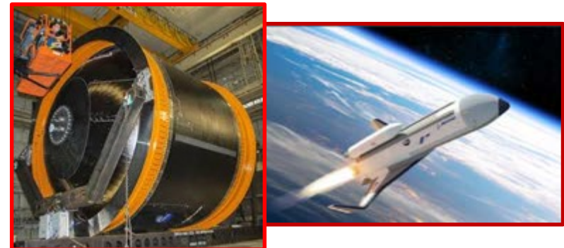
Boeing XS-1 project will use STMD composite cryogenic tanks
