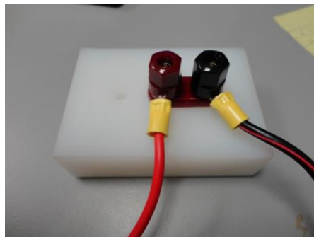
Figure 1: NBL Banana Plug Receptacle (electrical power)
