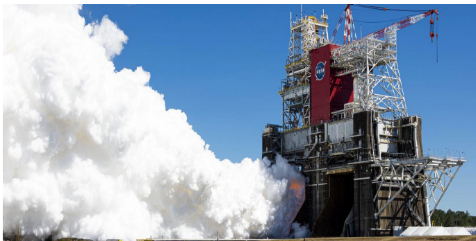
Artemis I core stage green run test in the B-2 test stand at NASA's Stennis Space Center in Bay St. Louis, Mississippi.
