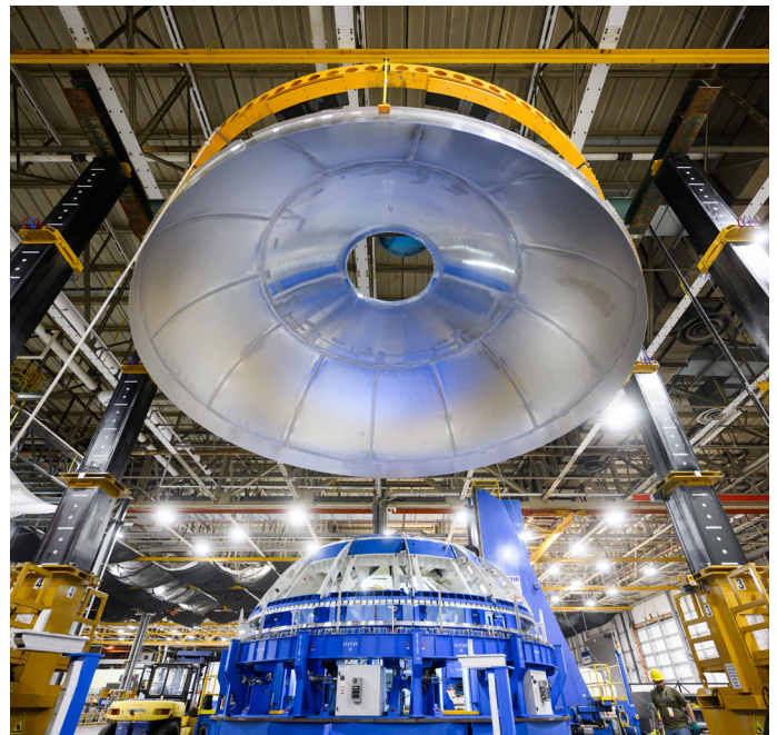
Technicians at Michoud remove from a robotic welding tool the dome for a liquid hydrogen tank test article for the future exploration upper stage.
