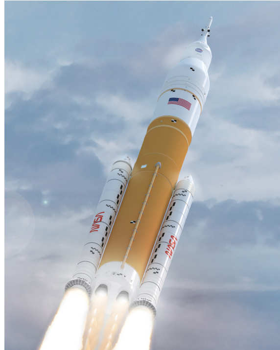
This artist's concept shows NASA's SLS (Space Launch System) in its Block 1B crew configuration.
