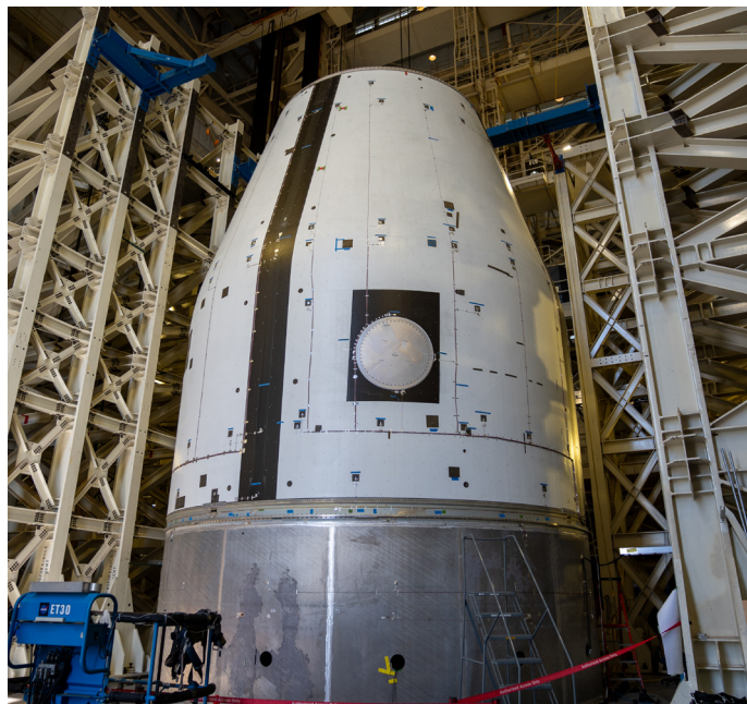
A test version of the SLS Block 1B universal stage adapter is moved into a test fixture at NASA's Marshall Space Flight Center in Huntsville, Alabama, to be subjected to simulated launch stresses. When Block 1B debuts on Artemis IV, the adapter will be capable of co-manifested payloads up to 10 metric tons (22,046 lbs.) and more than 10,000 cubic feet (283 cubic meters).
