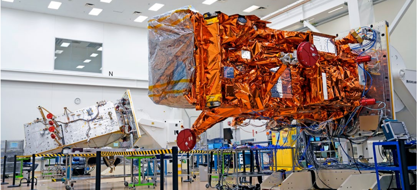
Next in the series after NOAA-21, the JPSS-3 (foreground) and JPSS-4 (background) satellites are being assembled and tested at the Northrop Grumman Spacecraft Facility in Gilbert, Arizona. CREDIT: NORTHROP GRUMMAN
