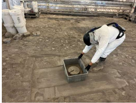
Figure 2. A team member using the bin-and-weight compaction method in a crosshatch pattern.
