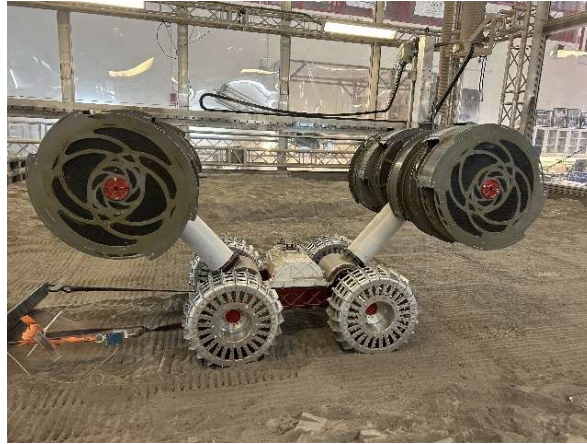
Figure 4. RASSOR 2.0 with its arms positioned at a 45° angle from the horizontal position.
