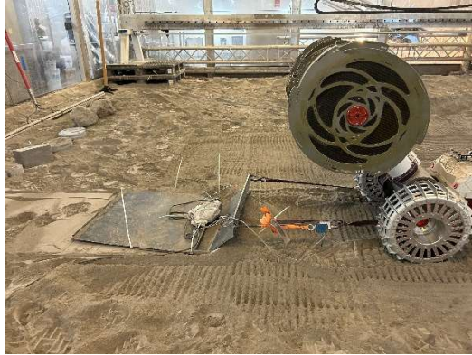
Figure 6. RASSOR 2.0 with a sled and attached load cell affixed to its back wheel hubs.
