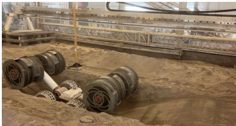
Figure 5. RASSOR 2.0 positioned at the bottom of the inclined surface before a slope test.
