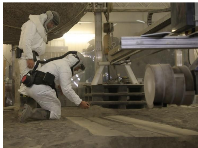
Figure 10. Team members taking geotechnical measurements of the Bucket Drum Test Bed following a test run
