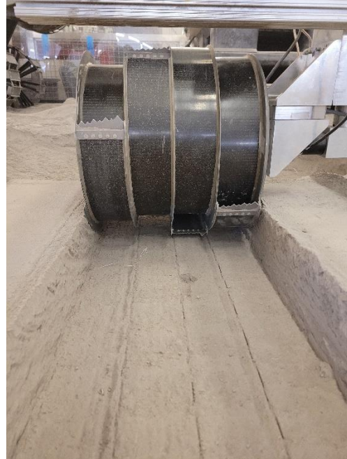
Figure 7. Bucket Drum Test Bed being precision leveled
