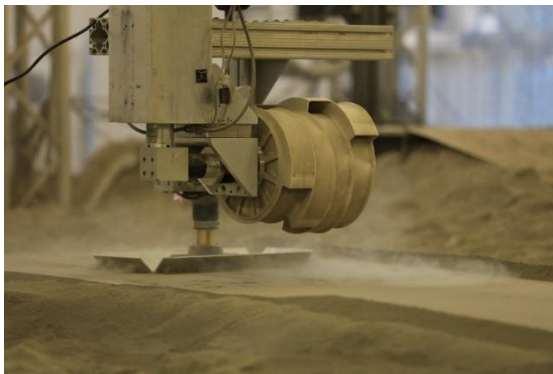
Figure 9. Bucket Drum Test Bed being precision compacted
