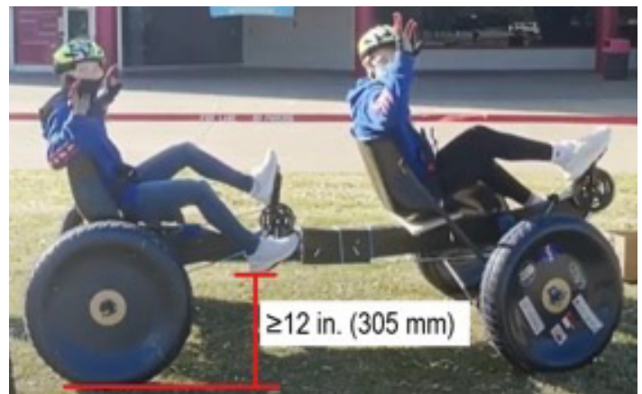
Figure 1: Vehicle Height Requirement.
